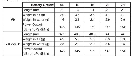
Stated tag length, weight and output power are nominal. Small manufacturing variations can be expected. Please contact VEMCO sales for details on V9T temperature tag weights and lengths.
