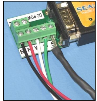
Flying Lead connected to terminal block
