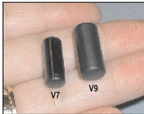
The V7-1L pinger has approximately half the volume and half the weight of the V9-6L pinger. This is particularly noticeable in the side-by-side comparison shown in the photo above.
