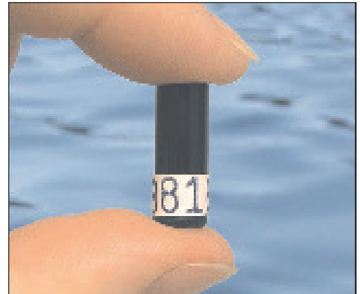
The V7-1L weighs only about 0.7 grams in water and is only 18 mm long.
