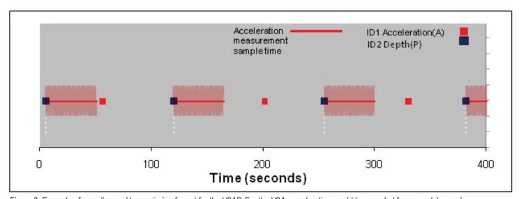
Figure 3: Example of sampling and transmission format for the V9AP. For the V9A, acceleration would be sampled for every delay cycle.
