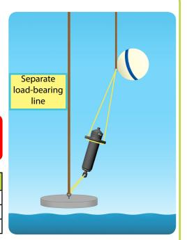
**NOTE: Safe Working Load (SWL)** sometimes stated as the Normal Working Load (NWL), is the maximum safe force that a piece of lifting equipment, lifting device or accessory can exert to lift, suspend, or lower, a given mass without fear of breaking.
