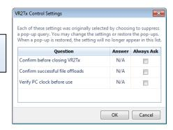
Changing an action is also possible in the Control Setting window, without enabling the query. For example, if "No" was selected when the "Import offloaded files into database" was disabled and you now want to import the data without being queried each time, then click the drop-down menu next to the answer and select "Yes" from the list.
