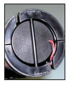
Downward force (see red arrow) may be required on battery end to get the pin started.
