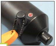
The flash pattern in a VR2Tx indicates the mode (state) the receiver is in at the time. A bright, long red flash once a second indicates that the VR2Tx is now ready for wireless communication but is not yet in communication with VUE.
