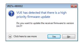
2. Has all the data been offloaded from the VR2Tx? If you are making a major update (e.g. from version 1.x.x to 2.x.x), then all the data in the receiver will be erased. Making a smaller update (e.g. from 1.x.2 to 1.x.3) should not erase the data, but please take the precaution of offloading all data before updating.
