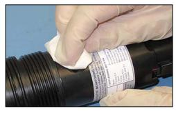
Place the receiver on a clean surface so the O-rings remain debris and damage free.
