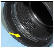
It is vital that all O-ring surfaces are clean and damage free or water may work its way inside the case and destroy the electronics within the VR2Tx receiver.
