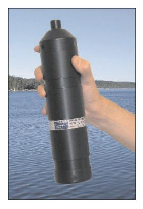
receiver range. Depth, temperature and other sensor data can also be collected. After removing your VR2Ws from the water, data is downloaded quickly and easily in the field without opening the case by using your PC with Bluetooth<sup>®</sup> wireless technology. The VR2W system uses VUE software that is compatible with Windows XP SP2, VISTA or Windows 7 operating systems.
