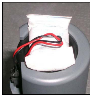
Desiccant pack in place
