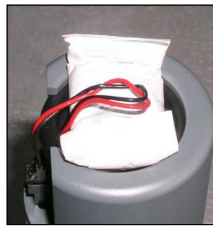
Desiccant pack in place
